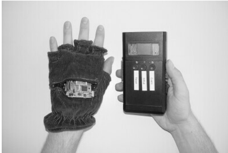
Figure 1: The sensor system consists of a glove containing sensors for skin resistance, skin temperature, ambient air temperature, and a heart rate data receiver; and a base unit processing, storing, and transmitting the data to a host.
