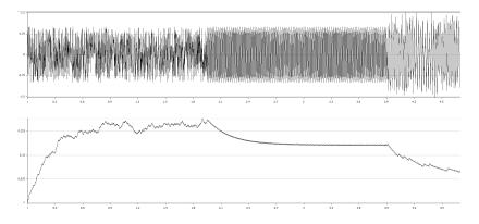
**Fig. 2.** This figure shows the momentary frequency estimation for a signal containing two transients, from white noise to a pure sinusoidal wave and then to a sine wave with a different frequency superimposed with white noise.
