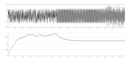
Fig. 3. This figure shows the momentary frequency estimation for a signal containing two transients again. This time the third part is a superposition of the white noise from part 1 and the sine from part two. As a result the white noise is filtered entirely.
